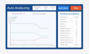
Titration speed can be set from 0.05 ml/s to 1.0 ml/s, with a minimum titration volume of 0.2 µL/step.
