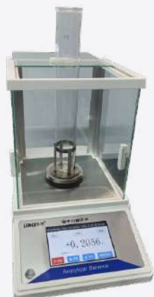
Electronic analytical balance with WIFI interface board installed and dedicated test tube weighing support.
